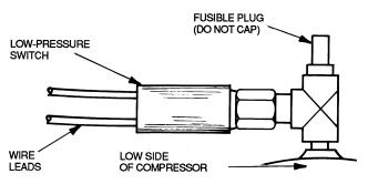
NOTE: 38AKS024 has a fusible plug in the liquid line.
